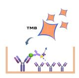
4、Add 100μL Substrate Reagent. Incubate for 15-20 min at 37°C
