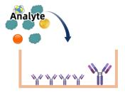
1, Add 100µL standard or sample to the wells. Incubate for 90 min at 37°C. Aspirate and wash plate for 3 times
